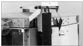
Installing screws in the rear lid brackets
