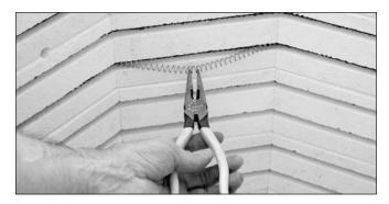
Remember, if you do not push the element fully to the back of each corner, the element will not stay in the grooves when fired.
