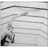
Using a propane torch with push button igniter to heat a bulging element.
