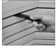
against the heat shield. They protect the element from contact with the case and heat shield, so they must not work their way out after the element connector is tightened into place.
