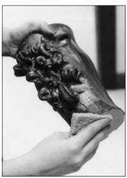
To dry foot a piece, remove all glaze from the portion of the piece that will rest on the shelf.
