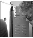
Wear firing safety glasses when looking through a peephole into a hot kiln.
