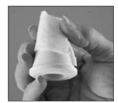
If a peephole plug falls out of the kiln, wrap it with a small piece of ceramic fiber paper. That will hold it in place.
