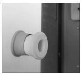
Keep the peephole plugs inserted if your kiln has a motorized downdraft vent.
