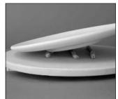
Separating the plate from the shelf helps to prevent cracking of the ware
