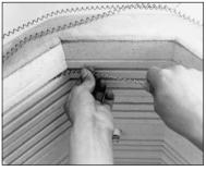
hold it with both hands in such a way that you are applying constant pressure that pushes the element into the corners. If you let go before the element is completely threaded, it will spring back out of the corners.
