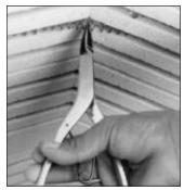
Expanding coils with automotive snap-ring pliers.
