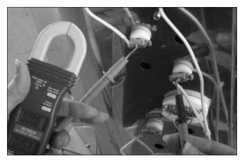
from one of the connectors. Otherwise current from the ohmmeter battery can pass through other elements than the one you are testing, causing an incorrect reading. Hold the element connector with locking pliers as you remove the screw. Be gentle to avoid breaking the element. (Elements are brittle after being fired.) Do not disturb the screw holding the element, only the one holding the lead wires. Reconnect the wires securely after testing the element.
