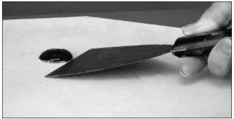
Hold the putty knife at a sharp angle to remove glaze from a shelf.
