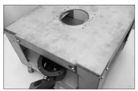
Installing the Orton Vent Master. The fan and fan housing are separate from the air intake cup shown above. The intake cup slides into the flange supports in the top of the kiln stand.
