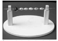
Separate the glazed beads so they do not stick together on the bead rod.
