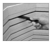
**Note:** Don't force the element into the groove corners. If the element won't fit easily, lengthen it with automotive snap-ring pliers (available from auto parts stores). Stretch the space between the
