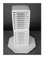
Tile holders are a special type of kiln furniture. They make efficient use of kiln space and allow air to circulate around tiles for even heating, thereby reducing tile warpage and cracking. Tile holders can be stacked inside the kiln.
