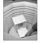
posts since short posts in the bottom of the kiln are more stable than tall ones. But if you have difficulty reaching down into a deep kiln, leave the bottom shelf in place and load tall pieces onto it. A short stepladder or concrete block is an aid to reaching into a deep kiln.
