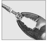
Squeeze a loose connector to tighten, but replace connectors that have been damaged by heat.
