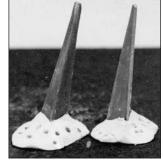
Standard large cones in clay cone packs.
