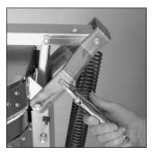
4 If the lid still rises during firing after all the above checks out okay, insert a screwdriver between each rear lid bracket and rear Litelid arm. Twist the screwdriver to ease possible binding. Or use locking pliers such as Vice Grips to bend the metal to remove binding. Or bend the yoke with your hands. When binding is removed, the lid will float again.
