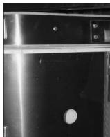
The light around the edge of the lid and inside the peephole changes color as the kiln gets hotter. You can learn to estimate temperature by the color of that light.
