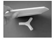
pends glazed ware on the wire points to separate the piece from the kiln shelf. Stilts also allow air to circulate around large, flat pieces. Stilts are needed for glazed ware, not greenware.
