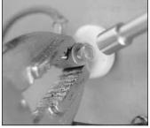
Tightening the element connector.
