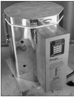
You can buy the galvanized sheet metal from a hardware store. It should be large enough to protect the entire kiln bottom.
