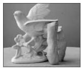
Rolls of porcelain clay are used here to support a delicate piece.
