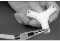
Straighten stilt pins with pliers.
