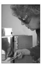
**Caution:** Some ceramists blow into the peephole to momentarily darken the cone so they can see it better. Please do not do this. This can blow brick dust onto the ware and is a safety hazard. Cool air also changes the temperature at which the cone bends.
