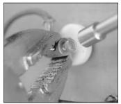
**5** Remove and save the Removing element connectors. porcelain insulators
