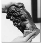
To "dry foot" a piece, remove all glaze from the portion of the piece that will rest on the shelf.
